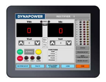
The Touchscreen Controller comes built into a standard remote console, allowing for flexible controller placement. Custom control placement options are also available on request. It can also be retrofitted to existing Dynapower power supplies or SCR units supplied from other manufacturers.
