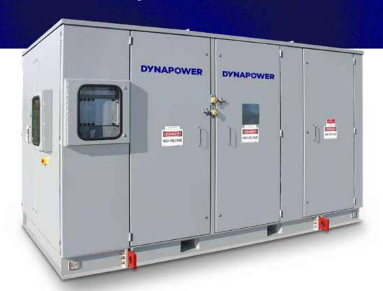
IGBT Chopper rectifiers are designed for high power factor and low harmonic distortion, eliminating the need for power faction correction equipment and harmonic filters. They also have inherently low ripple (typically <2%) at full output so ripple filters are not needed.
